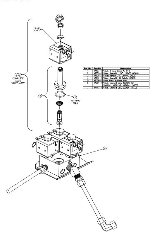
Figure A.5: Valve Block Assembly
