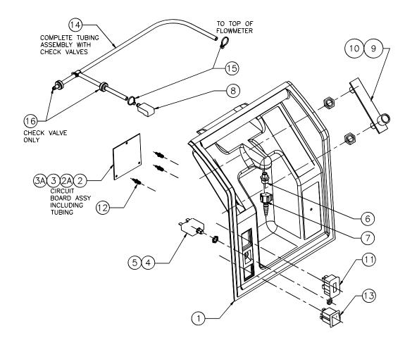
Figure A.1: Control Panel Assembly
