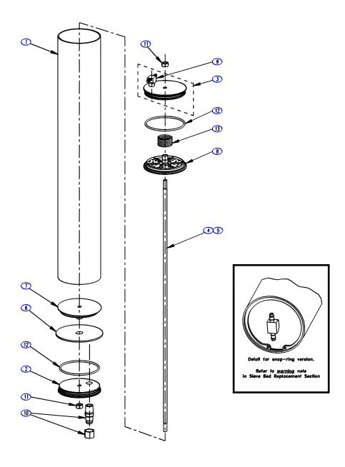
Figure A.7: Adsorption Bed Assembly
