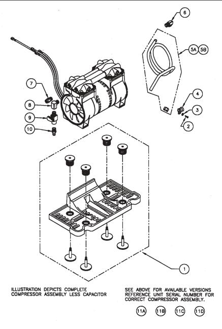
Figure A.6: Compressor Assembly
